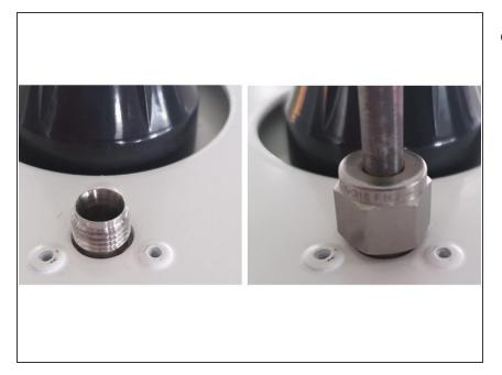
Attach the inlet using a ¼ inch Swagelok compression fitting.
