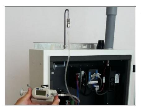
Perform a flow check to make sure the inlet is fitted correctly and the sample pump is working properly.
