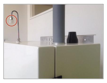
Fit the supplied Kynar fitting to the Swagelok nut at the end of the sample cane. This fitting contains the mesh filter.
