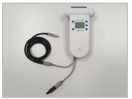
If you have a temperature and relative humidity sensor, first connect the two-way PS2 adapter cable that came with your Series 500 to the RS 232 port on your monitor.
